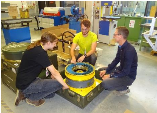
Caption 5: In the WARR Hyperloop capsule a turbine minimize the resistance and the friction in the partial vacuum.
